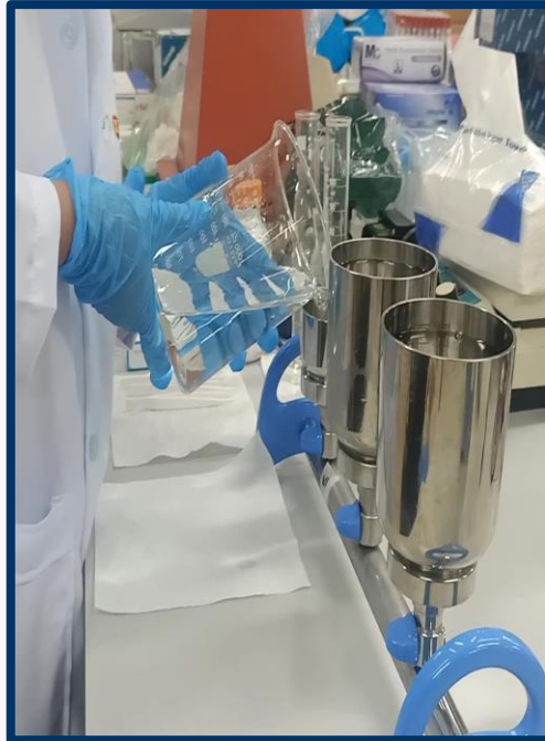
Figure 8. Filtration using glass microfiber filter papers (0.7 \mu m pore size)
