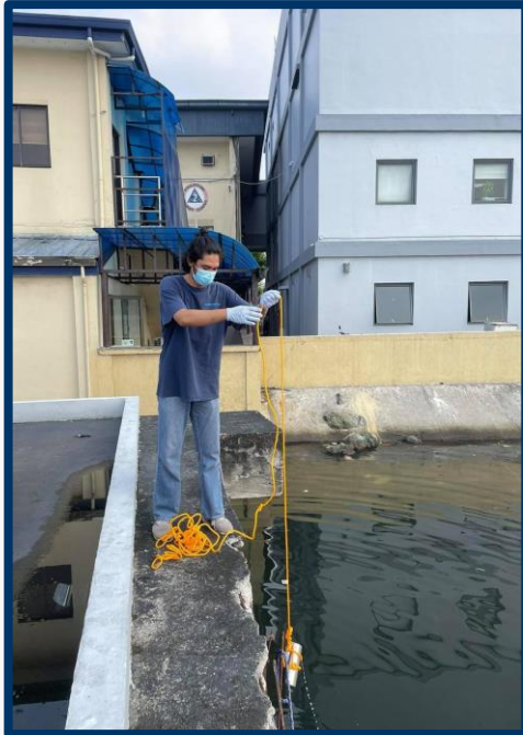
Figure 7. Water collection of two litres with replicate from port
